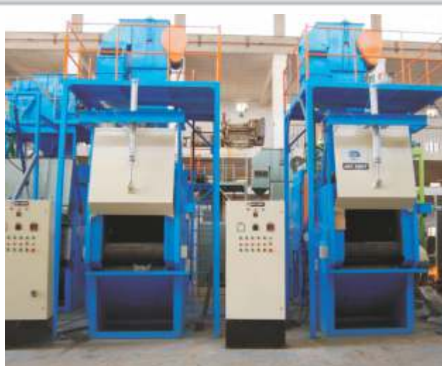
ATB 27" x 36" with Pneumatic Control Door
