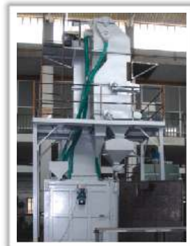
Airless 2W Hanger Type Blasting M/c for Automobile Industry with Magnetic Shot Separator
