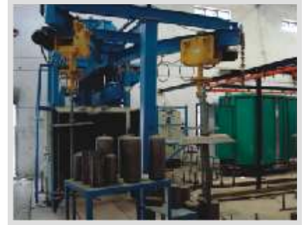
Airless 'Y' Hanger Type Shot Blasting M/c for Fire Extinguishers
