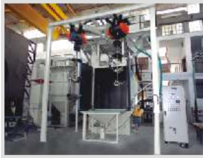
'Y' Hanger Type Shot Blasting M/c with Motorized Hanger for Valve Bodies
