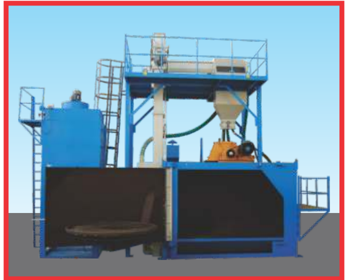
Airless Shot Blasting Machine Swing Table Type MODEL AST-1800
